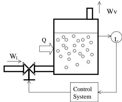
Figure 6. Schematic diagram of simplified steam generator model
